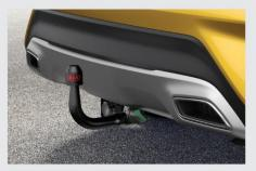
KUKA ZA VUČU - MONTAŽNA
